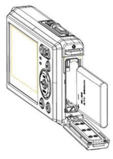
3: After the battery is properly installed, replace the battery cover until an audible click is heard.
