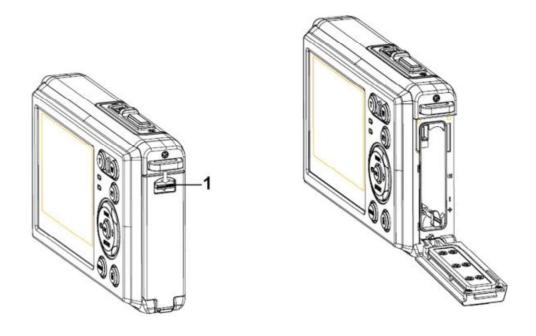
2: Insert the battery with the positive (+) and negative (-) terminals matching the direction indicated inside the battery compartment.
